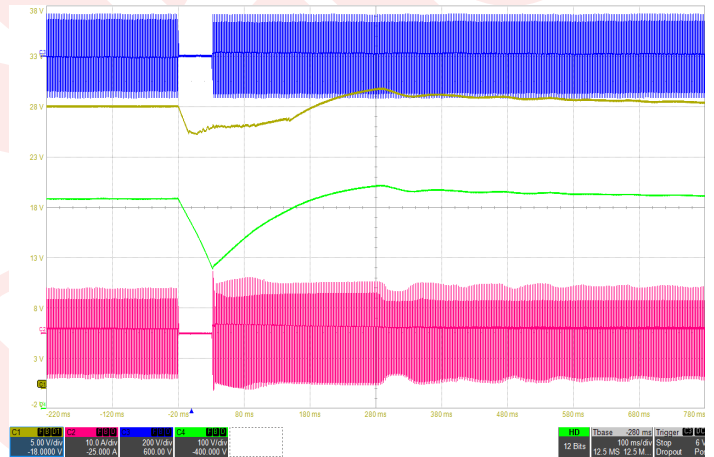
Figure 10: Line drop out with 600µF hold-up capacitor at full load (115Vrms, 400Hz) Ch1: Vout (5V/div), Ch2: Iin (10A/div), Ch3: Vin (200V/div), Ch4: Vhold-up (100V/div), Timebase: (100ms/div).
